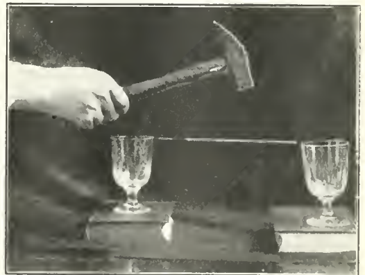
FIG. 2. AN EXPERIMENT IN THE FORCE OF INERTIA
